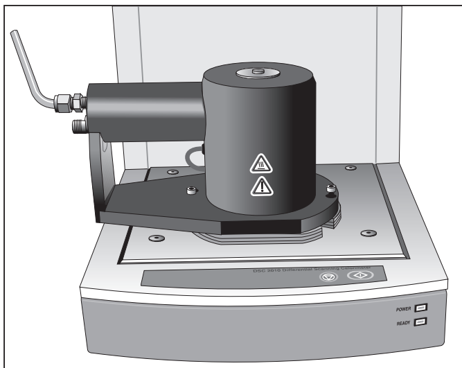
Figure 2.6 DSC Cell Heat Exchanger Assembly on the DSC 2010 CE
