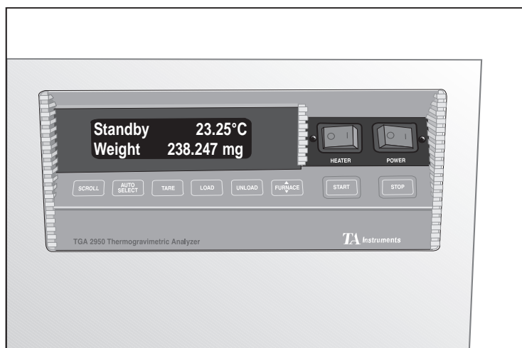
Figure C.2 TGA Instrument Display and Keypad with Auto TGA Accessory
